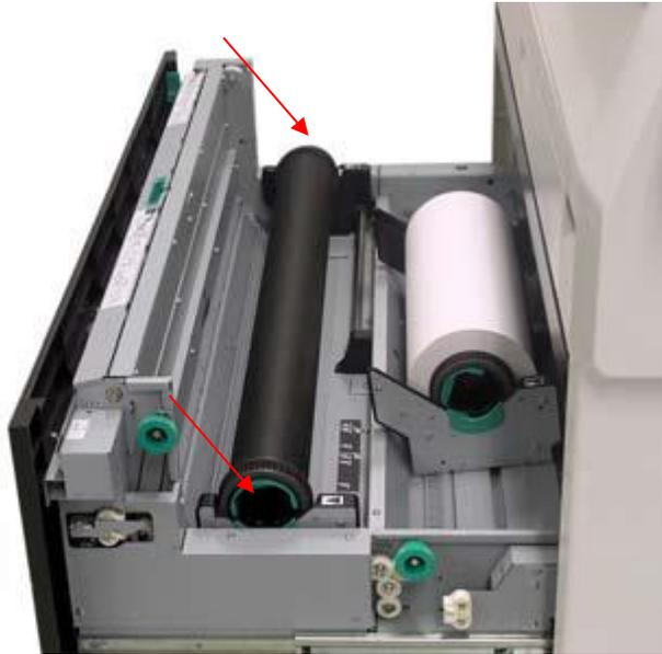
3. Raise the green lever and remove both Flanges. Set aside for Step 5.
