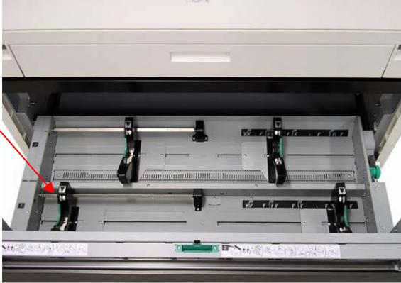
5. Insert each Flange into both ends of the new roll to be installed (removed from Step 3). Push both the green levers down so they are flat against Flange.
