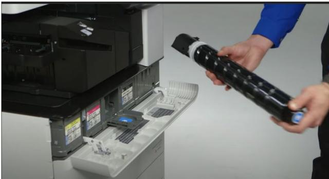
3. Open the new cartridge and insert into the designated slot of the machine
