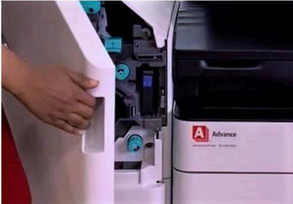
2. Remove the staples cartridge from the cartridge carrier (Green Tab)
