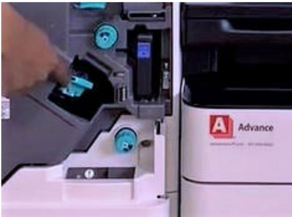
3. Press on both sides to remove the cartridge from the casing
