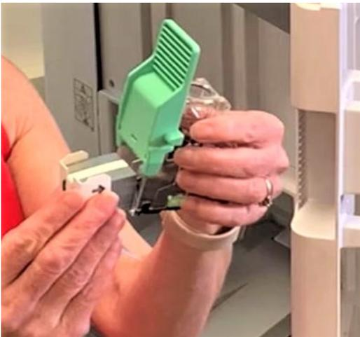
5. Insert the staple cartridge into the cartridge carrier
