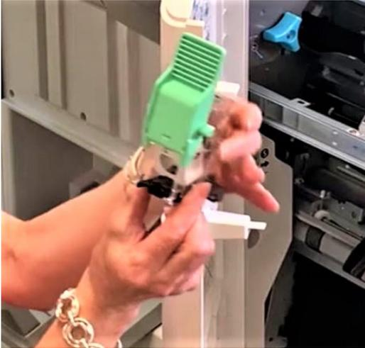
4. Insert new cartridge into the casing until it clicks into position
